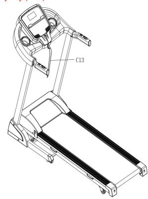
**Step 6:** To check if the running belt runs correctly, placing treadmill in folding position and tightening all the bolts. Then set speed under 3km/h and see if running belt runs without problem.
