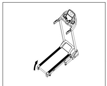
Lift up the machine and force to pull up until you heard "click" that made by safety casing stuck the pneumatic cylinder.
