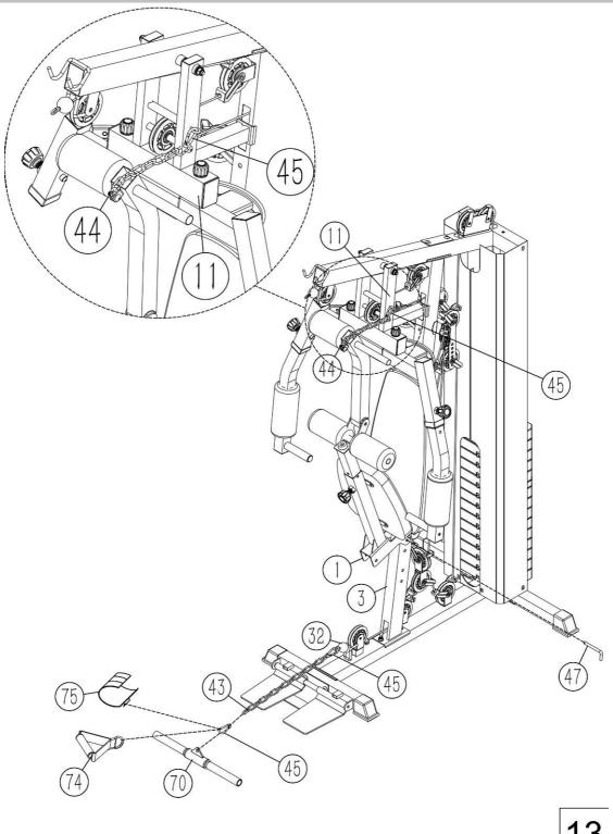
Fold the seat pad support as the diagram shows, you must fix the leg developer them as the diagram shows with 2pcs gourd hook(45) and one pc 8-joint chain(44) for safety ,Connect the shiver bar (23) or single strap(43) or angle strap(42) to the lower cable to do the desired exercise
