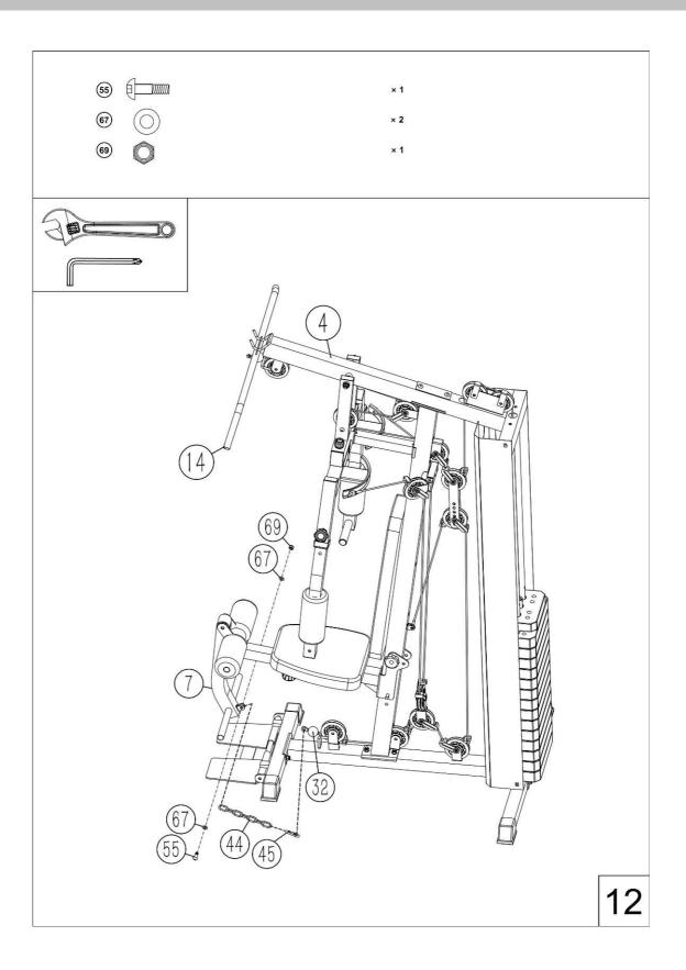
Connect the leg developer (7#) to the end of the lower cable with 1pcs gourd hooks(45), one pc 8-joint chain(44), one pc M10\*28 Allen bolt, 2pcs Ø10 washers(67) and one pc M10 Aircraft nut(69)
