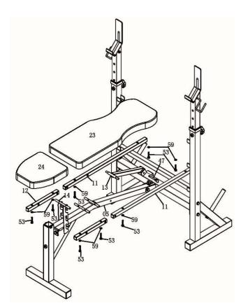
Attach the Seat Adjustment Bar (14) beams to the Seat Tube (12), at the same time attach the Seat Tube (12) to the Maine Frame (05) as illustrated. Attch the Seat to Seat Tube (12) using four Hex Bolts (53) and four Flat Washers (59).
