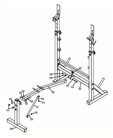
Attach both Left/Right Uprights (01 &02) to the Cross Bar (03) using four Hex Bolts (49),eight Flat Washers (58) and four Nylon Lock Nuts (56).
