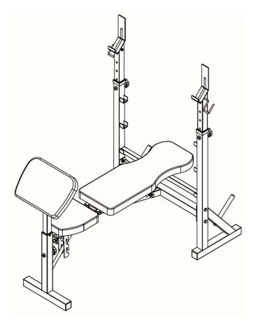
Attach Arm Curl (25) to the Arm Curl Tube (15) using two Flat Washers (59) and two Hex Bolts (54) .
