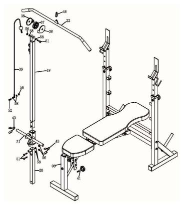
With Lat Tower Cable (39) in groove of Pulley(37).thread the Lat Tower Cable (39) through Lat Tower Tube Upper(19) bracket.
