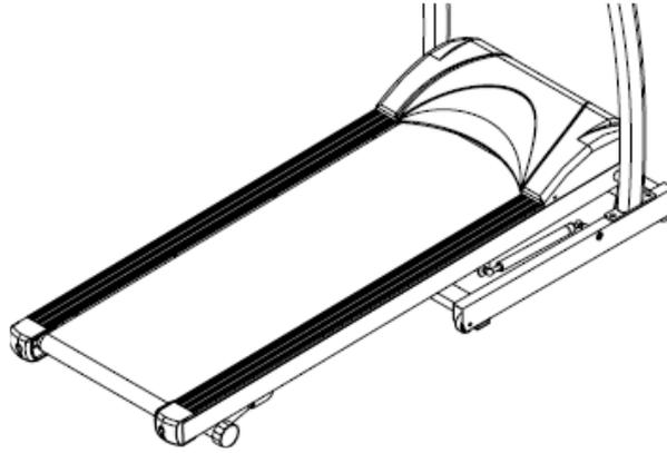
Right and left Allen bolts are located at the rear of the treadmill.
