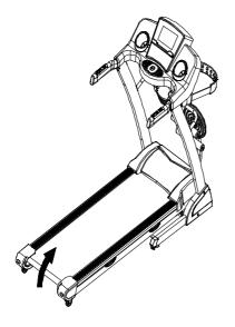
Lift up the machine and force to pull up until you heard "click" that made by safety casing stuck the pneumatic cylinder.
