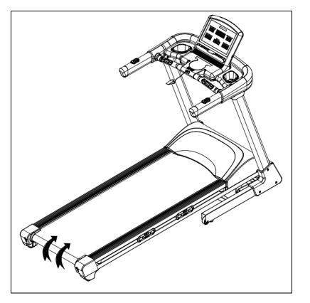
To fold up the treadmill: Both hands hold on the bottom end covers and lift up the treadmill.
